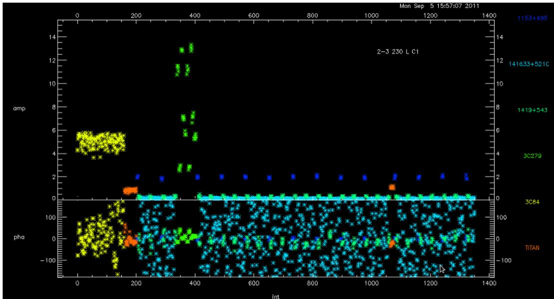
Figure 8. Amplitude and Phase vs Integrate time after flagging the Integrate time which larger than 1350.
